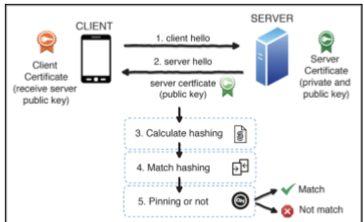
SSL Pinning implementation by means of certificate hashing By Apurv Pandey (mailapurvpandey.medium.com)
